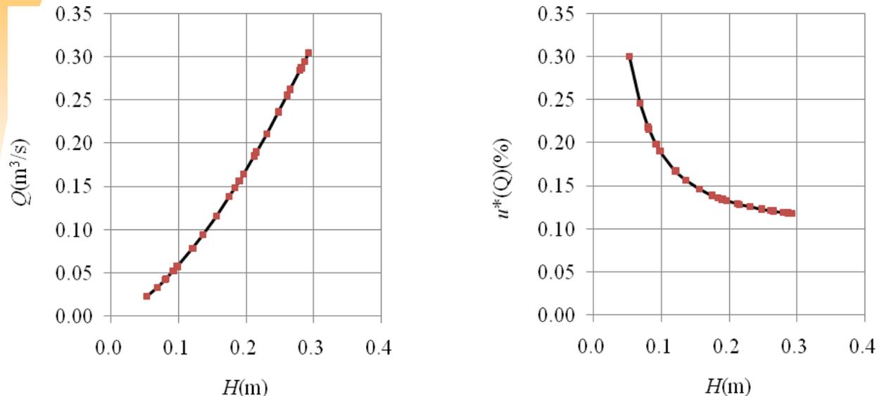
Figure 2. Curves of  $Q$  and  $u^*(Q)$  versus  $H$
