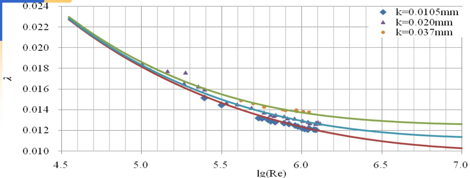
The above Figure shows the curves of  $\lambda$  versus  $Re$ , in which the discrete points are drawn by the measured data and the solid lines are computed by the Colebrook Equation at  $k=0.0105\text{mm}$ ,  $0.02\text{mm}$  and  $0.037\text{mm}$ , respectively. Obviously, except some positions in which there are the greater deviations when  $Re$  is less, the deviations between the measured data and computed one is less than 1% in most of the positions.
