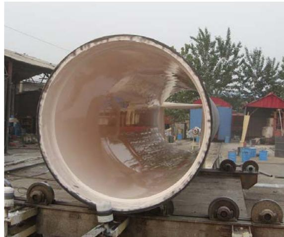
Polyethylene lining pipes
