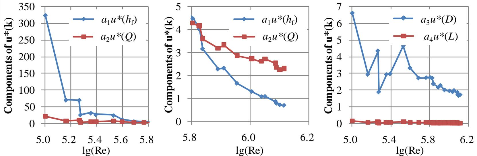
As mentioned above, one comes to a conclusion that for the ductile cast iron pipes lined with epoxy resin  $k=0.02\text{mm}$  and  $u^*(k)<5\%$ . Similarly, it is calibrated that if  $u^*(k)<5\%$ ,  $k=0.0105\text{mm}$  for the ductile cast iron pipes lined with polyethylene and  $k=0.037\text{mm}$  for the ductile cast iron pipes lined with cement mortar.
