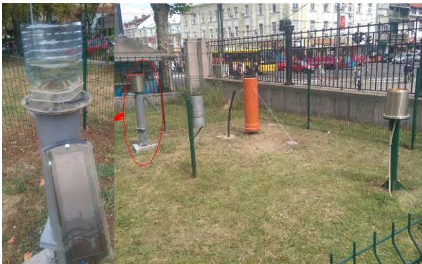
Figure 5. Meteorological area of the Belgrade Faculty of Civil Engineering (right) with Arduino based rain gauge (left)
