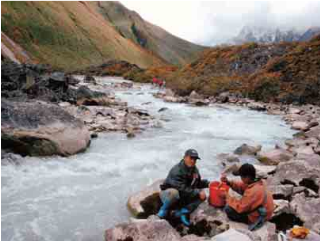
Photo 1: Preparing the salt dilution, Tarina II lake outlet (Bhutan)
