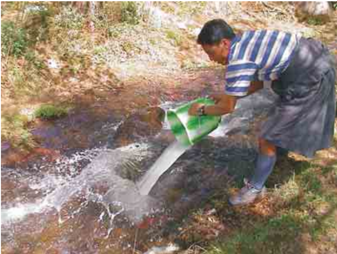
Photo 2: First bucket full of salt solution being injected into a stream, Bhutan
