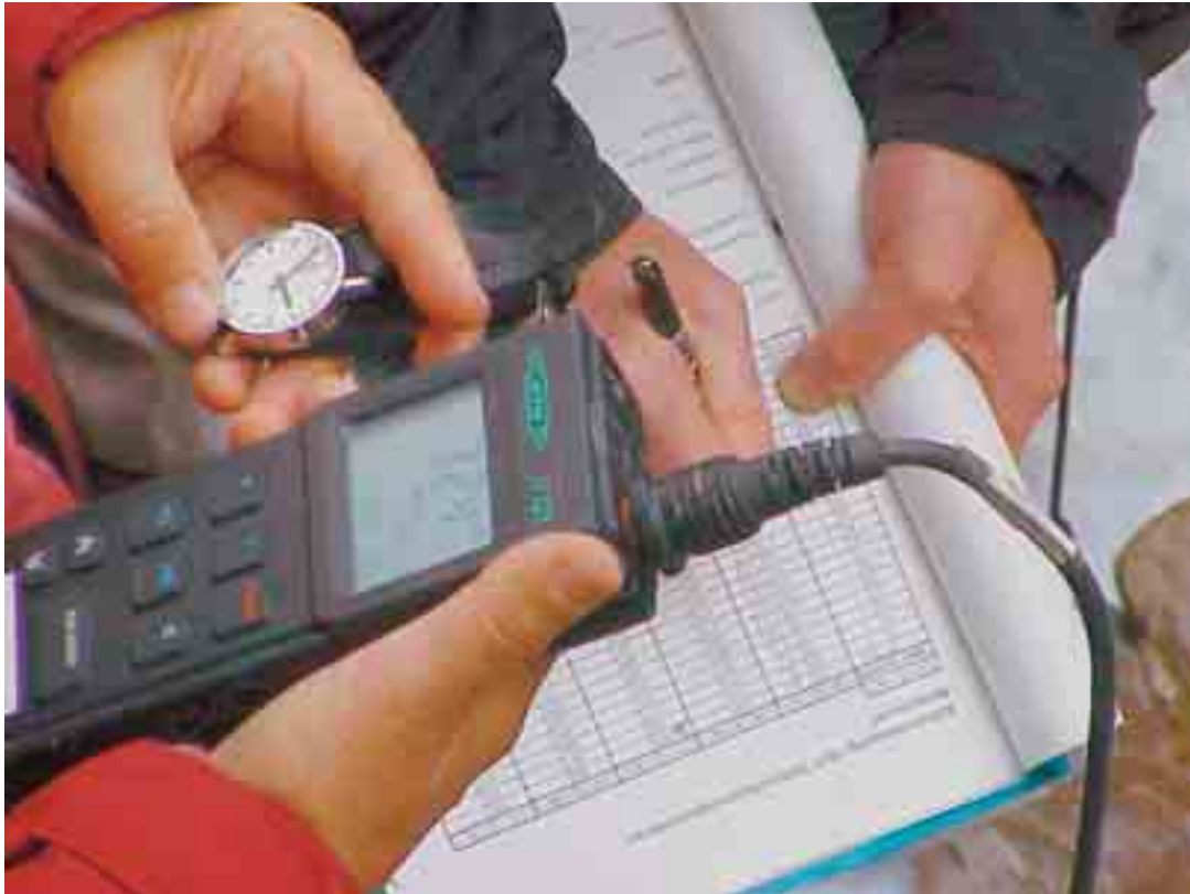
Photo 3: Taking conductivity readings every five seconds
