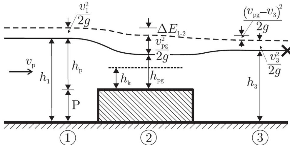
$$P + h_{pg} + \frac{V_{pg}^2}{2g} = h_3 + \frac{V_3^2}{2g} + \frac{(V_{pg} - V_3)^2}{2g}$$
