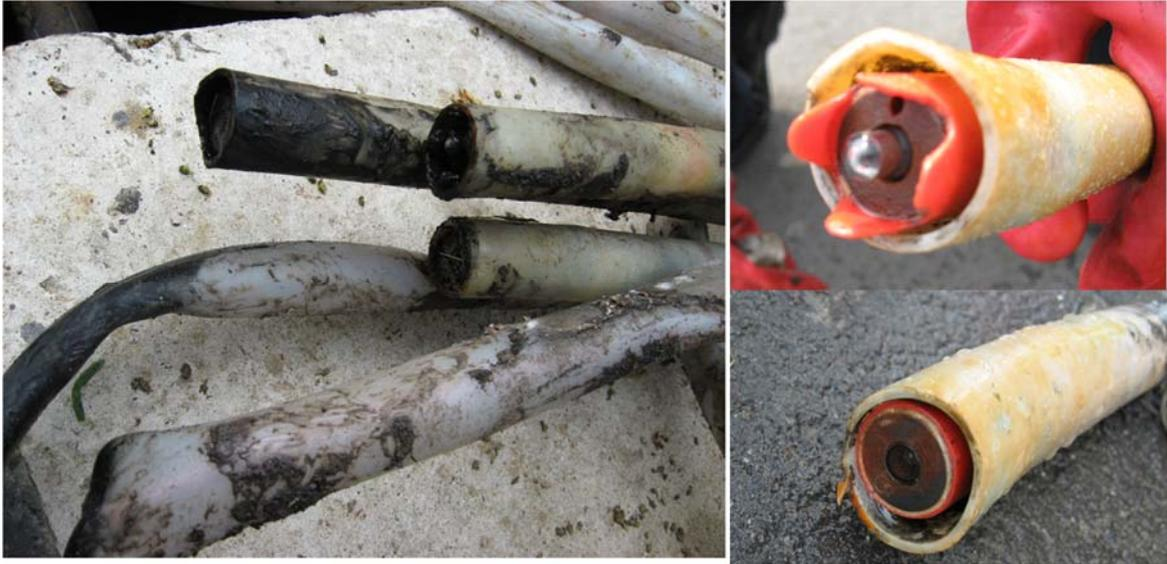
Figure 6. Probe for continuous measurement – before cleaning (left) and after cleaning (right)
