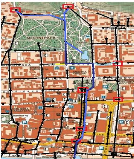
Figure 10. Recommendations for sewers along Svetozarevska street: new sewer from existing overflow to the pond in the city park, redirect flow to neighbouring retentions and construction of new retention
