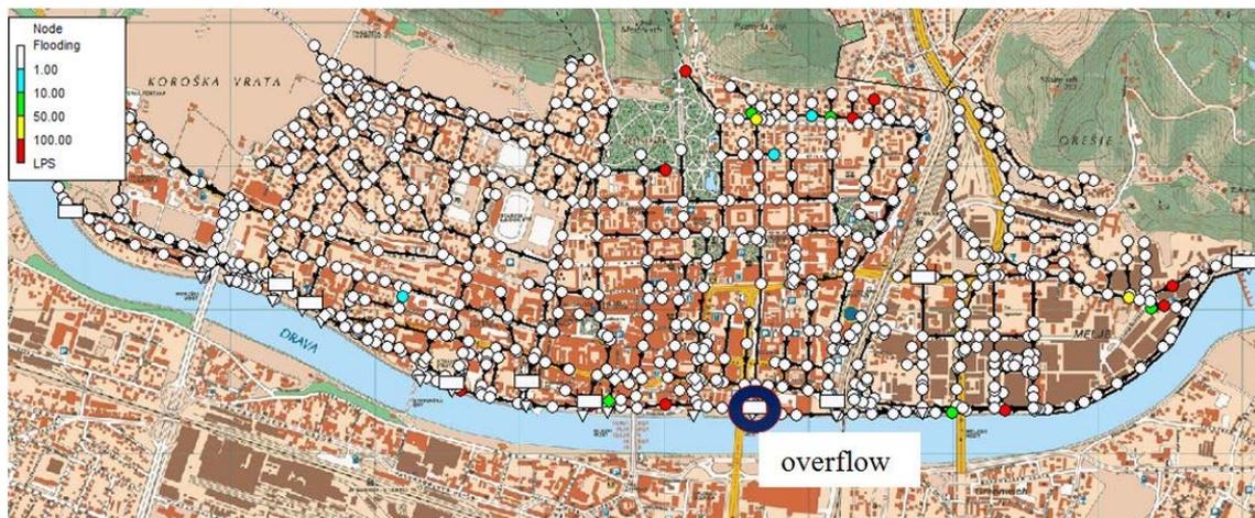
Figure 5. Simulated flooding at nodes (in lps) at the Drava river left bank based on SWMM due to 20 min. and 20 % probability design rainfall and surcharged CSO
