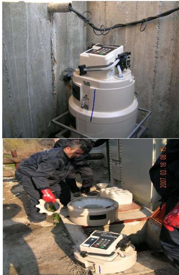
Figure 7. Automatic sampler
