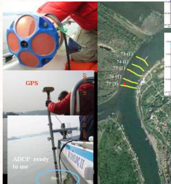
Field measurements at the confluence of Sava and Danube Rivers for 3D model validation
