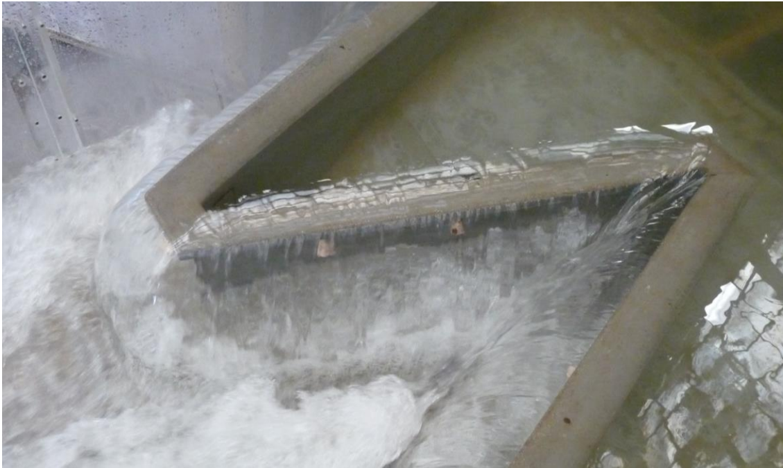
Hydraulic model of a labyrinth weir: Institute for the Development of Water Resources „Jaroslav Cerni“. Photo: R. Kapor
