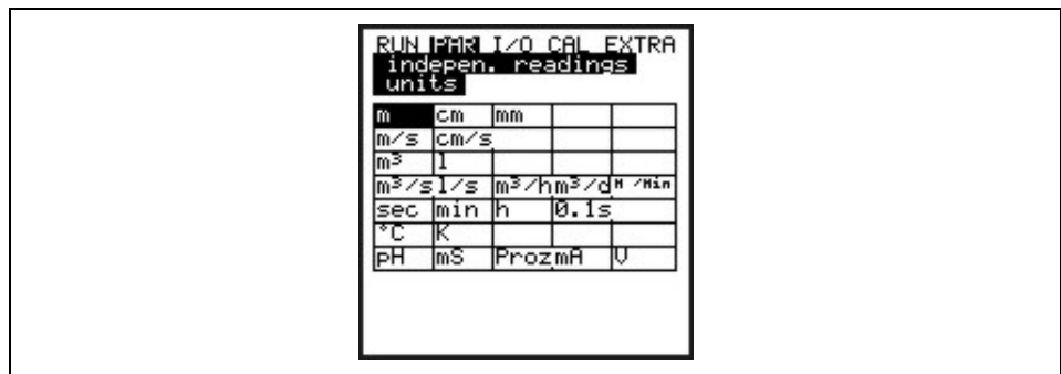
Fig. 8-79 Units of independent readings
