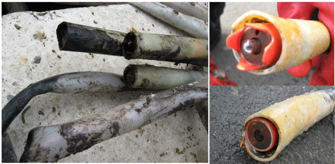
Figure 6. Probe for continuous measurement – before cleaning (left) and after cleaning (right)
