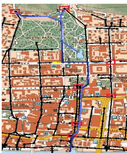
Figure 10. Recommendations for sewers along Svetozarevska street: new sewer from existing overflow to the pond in the city park, redirect flow to neighbouring retentions and construction of new retention
